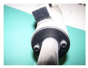
the snap ring that retains the rod guide. Items that should be at hand are a vise, flat punch, hammer, rubber hammer, clean oil, clean paper towels or shop towels and a wrench for removal of the piston nut. A piston ring compressor would be useful but is not necessary for resizing the teflon piston seal.
